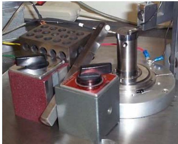
Figure 10: Dynamic Stiffness Test Setup
